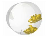
DEM based computer simulations were used to evaluate the performance of the chips seasoning and the device. The effects of various process parameters on the seasoning performance were determined. The study helped in reducing variability by over 50%
